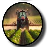
A rational application of pesticides and herbicides, applied at different times, using spray booms that are properly monitored for nozzle wear, pressure gauge functionality, and anti-drip device, and equipped with a suitable filter for proper sealing. These operations require proper adjustment of the spray boom.
