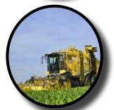
The harvesting process involves trimming, uprooting, removing excess soil, and loading the beets onto a machine for storage in suitable containers, followed by direct unloading onto trailers or trucks.
