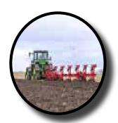
The main tillage is carried out to a plowing depth of 40-50 cm, to maximize the use of rainwater accumulation; this operation is performed simultaneously with the incorporation of crop residues and organic fertilizers by turning the tilled soil.
