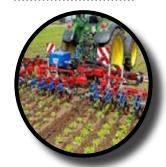
Hoeing the soil with hoeing machines equipped with special rotating tools or small earthing tools, similar to plow bodies, which carry out the operation of returning a portion of the soft surface soil towards the plant.
