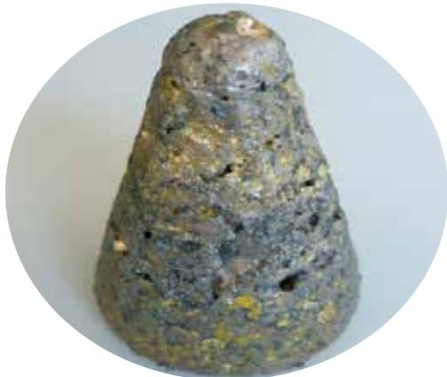
We will obtain synthesis gas treating the organic fraction in a **plasma torch**. The inorganic fraction becomes completely inert and forms a vitrified material. Then, pouring from the reactor in molten form (lava), it cools down solidifying in a material that can be shaped and used for useful purposes without environmental risks such as:
